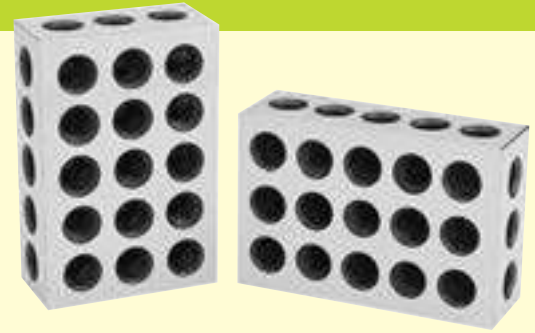
5 Tapped Holes & 18 Untapped Through Holes
